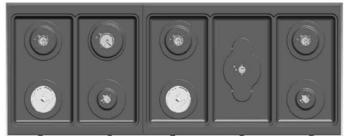
Dual Burner LPG: 1.27 - L20 NG: 2.38 - N21 Auxillary Burner LPG: 0.65 - L6 NG: 1.04 - N6 Dual Burner LPG: 1.27 - L20 NG: 2.38 - N21 Fish Burner LPG: 1.08 - L15 NG: 1.79 - N15 Auxillary Burner LPG: 0.65 - L6 NG: 1.04 - N6
