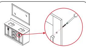
Remove the handles from inside the cabinet doors and drawers and reinstall on the outside. Do not over tighten when reattaching.
