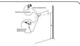
② Install the mirror: use a pencil to mark the placement of the screw holes on the wall, drill the holes and insert the plastic wall anchors.
