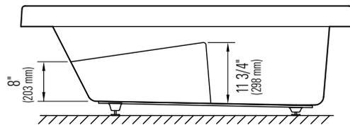
\*A bathtub fitted with back jets can cause the pump to protrude by approximately 3" from the overall dimension.
