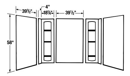
**General:** Furnish and install as shown on plans DURAWALL® Bathtub Walls, model 56, as manufactured by E.L. Mustee & Sons, Inc. The deluxe hi-impact Co/Poly wall system shall be five-piece construction with six formed shelves, and one-piece, seamless corner panels with overlapping edges and have uniform color throughout entire thickness. Color \_\_\_\_\_ (White, Bone).
