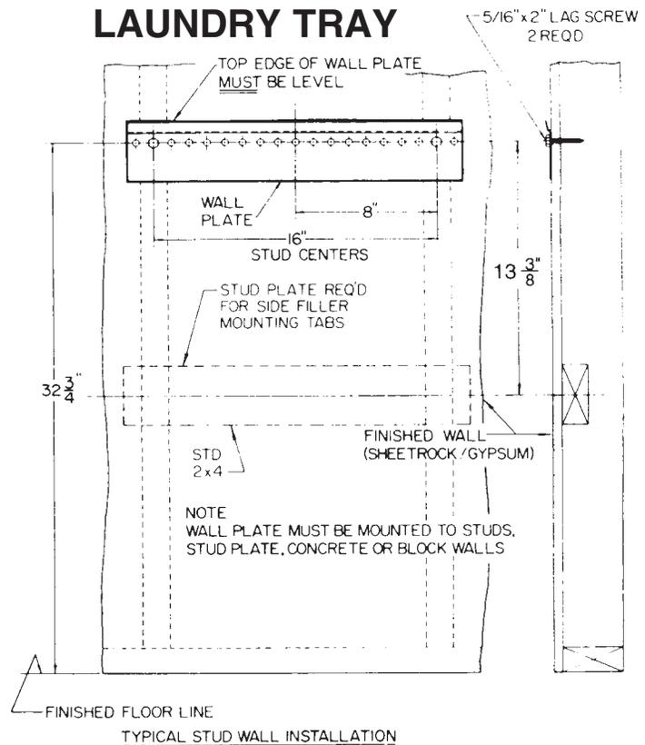
1. Secure **Wall Plate** to wall using both 5/16" x 2" **Lag Screws**. Locate mounting holes 1-1/2" below desired tray height as measured from top edge of rim.
